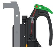
Half-span position of the trigger lodged in the upper handle
