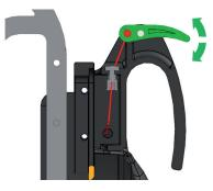
Start of trigger span position + indication of allowed pitch of few degrees (green arrows). The trigger is lodged in the upper handle
