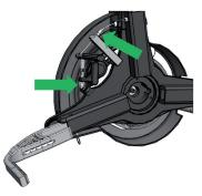
Rear view of the quick clamp + indication of the nut and locknut positions (green arrows)
